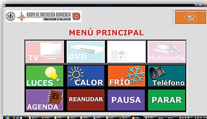
Figure 2. Main Menu of the domotic BCI application while running. In this frame the first row is highlighted.
